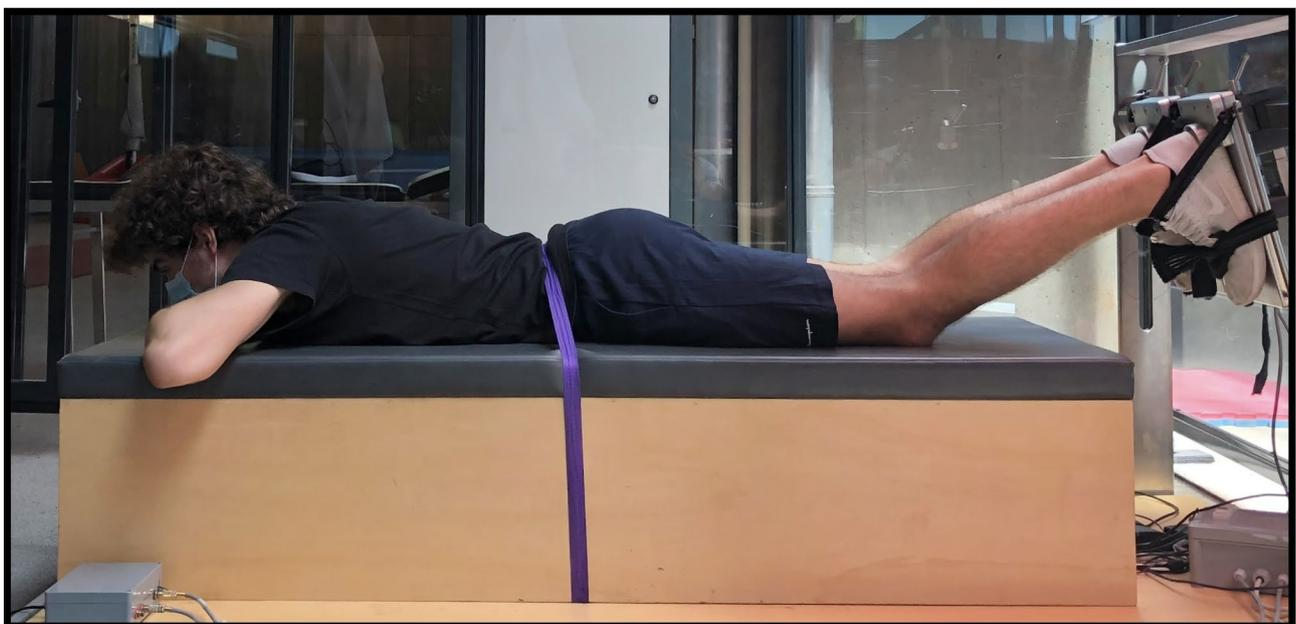
**Fig. 1** Experimental setup used to assess the knee flexors' peak torque and rate of torque development with 30° of knee flexion and neutral hip
