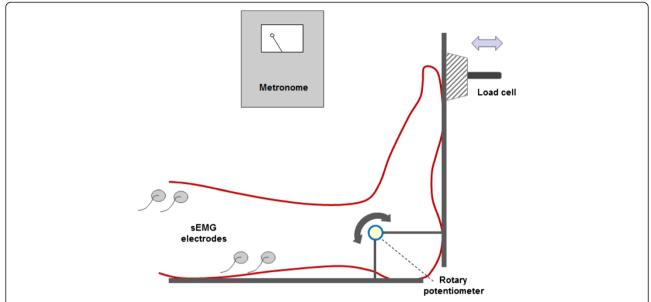
**Fig. 2** Experimental setup indicating footplate system with the lateral malleolus aligned to the axis of rotation of the rotary potentiometer. Surface electromyographic signals were recorded from the tibialis and soleus muscles. Oscillation of the footplate was synchronized with the audible beat of the metronome and the manually applied force was measured by the load cell
