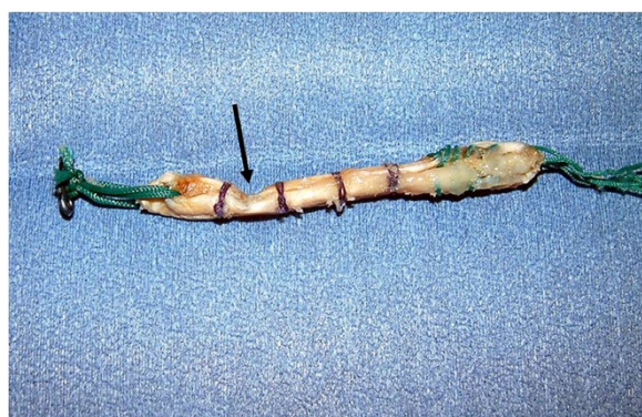
Figure 7 Graft deformation after 500 cycles of 0 to 100-N anterior tibial loads. Graft was deformed at the corner of the femoral tunnel aperture (arrow).
