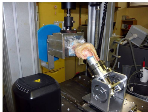
Figure 1 Photograph of the testing system with knee joint at 30^{\circ} of flexion.
