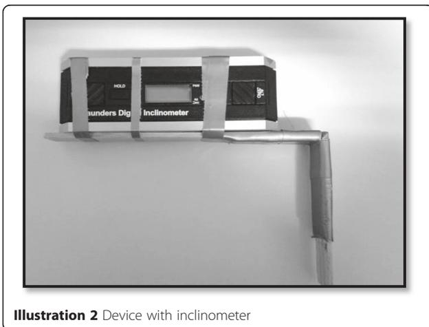
**Illustration 2** Device with inclinometer
